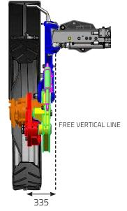
An extremely small front section to move between the rows without damaging them.
